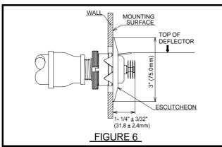
Do not continue to push on the Escutcheon such that it lifts a wall out of its normal position. If the Escutcheon cannot be engaged with the Sprinkler, or the Escutcheon cannot be engaged sufficiently to contact the back wall, relocate the sprinkler fitting as necessary.
