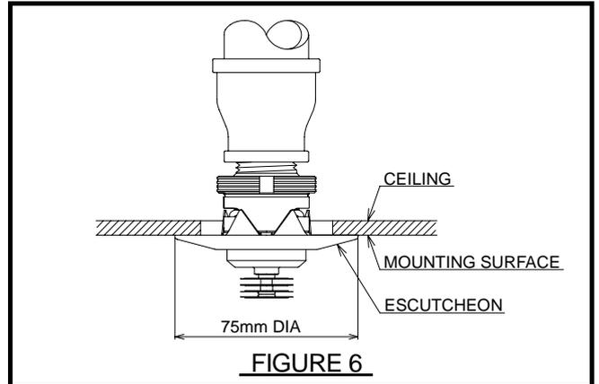
Do not continue to push on the Escutcheon such that it lifts a ceiling panel out of its normal position. If the Escutcheon cannot be engaged with the Sprinkler, or the Escutcheon cannot be engaged sufficiently to contact the ceiling, relocate the sprinkler fitting as necessary.
