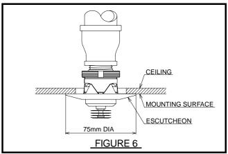
Do not continue to push on the Escutcheon such that it lifts a ceiling panel out of its normal position. If the Escutcheon cannot be engaged with the Sprinkler, or the Escutcheon cannot be engaged sufficiently to contact the ceiling, relocate the sprinkler fitting as necessary.
